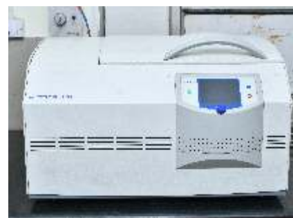
Cooling centrifuge for routine experiments related to molecular cell biology, chemical biology, proteomics and metabolomics
