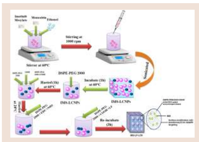
Synthesis of imatinib mesylate-loaded lactoferrin-modified PEGylated liquid crystalline nanoparticles for treating hepatocellular carcinoma
