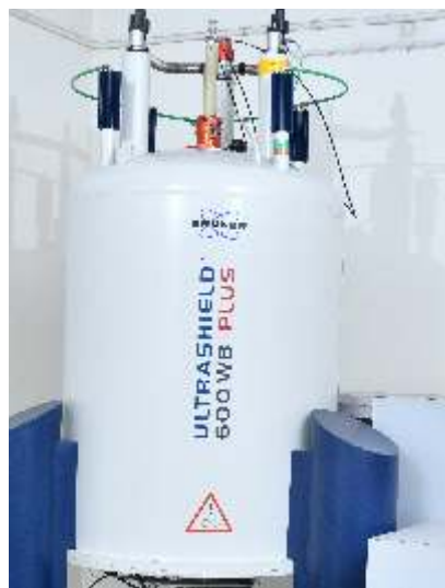
Bruker 600 MHz NMR Spectrometer for Solid state NMR of biological solid materials
