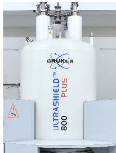
High field 800 MHz NMR Spectrometer for Solution state NMR and metabolomics studies.
