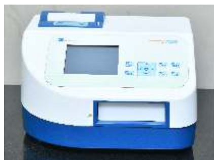
PCR machine for qualitative and quantitative estimation of nucleic acids in biological samples in addition to regular genome enhancing and DNA cloning related work
