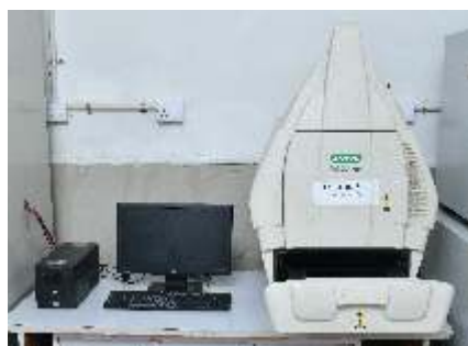
Gel Documentation System for visualization of DNA gels, image capturing and analyzing
