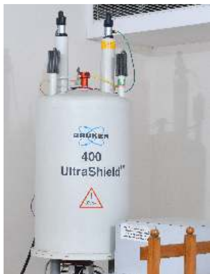
Bruker 400 MHz NMR Spectrometer for routine solution state NMR experiments
