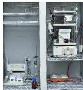
Fast Protein Liquid Chromatography (FPLC) for purifying recombinant proteins for elucidating their structures and studying their interactions using NMR.
